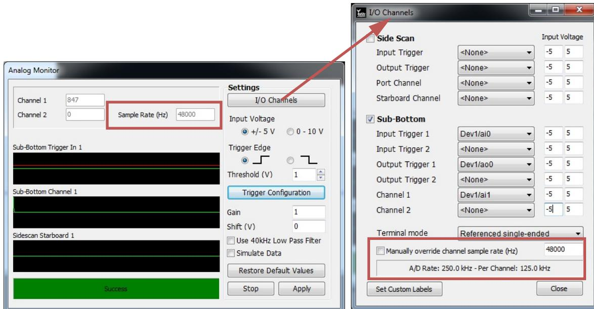
**Example 2: User-selectable sampling rates for a single channel sub-bottom profiler and two sub-bottom profilers collected simultaneously with internal triggers.**
