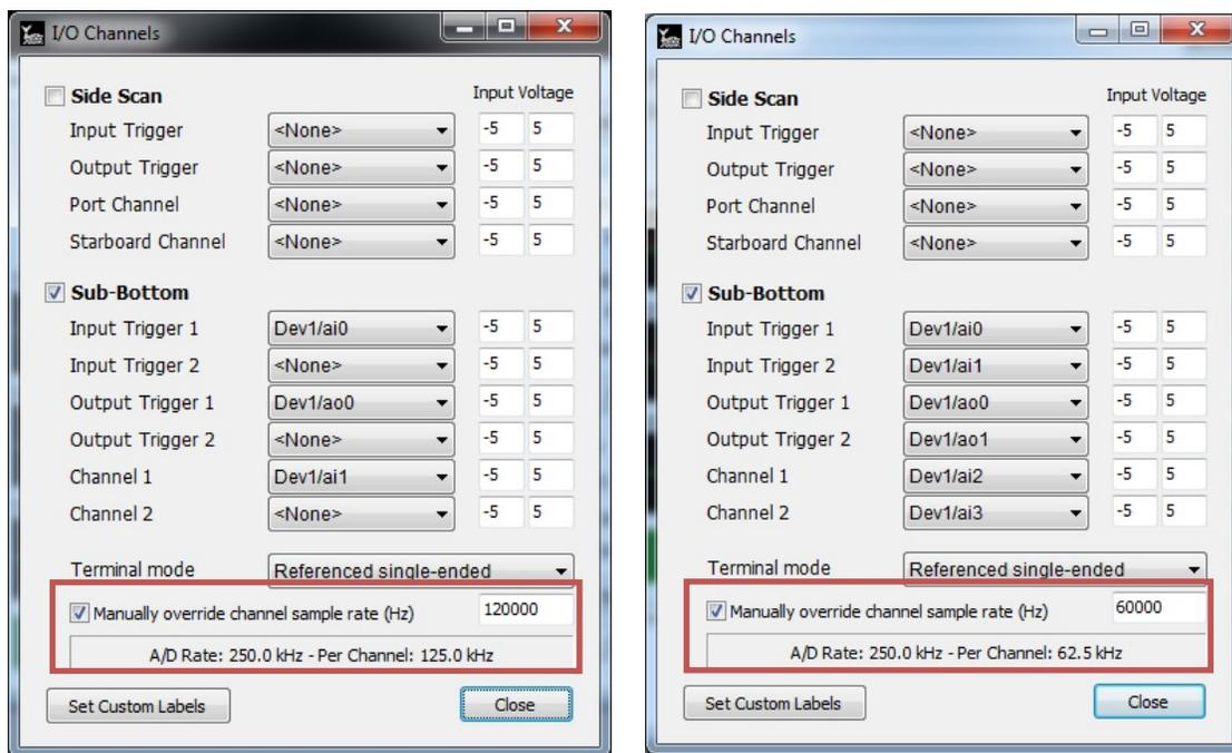
**Example 3: User-selectable sampling rates for a two channel side-scan and a single channel sub-bottom profiler collected simultaneously with internal triggers.**
