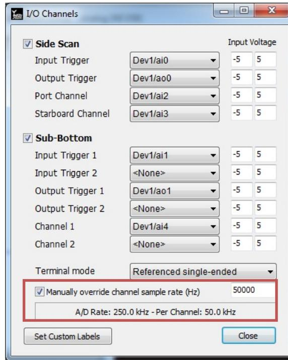
**FIGURE 4.** If too high a sampling frequency is selected for the type of NI-DAQ device and the number of channels selected, a “Queue is Full” message will appear in the Analog Monitor main window.
