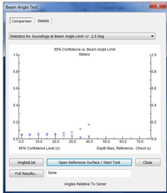
**FIGURE 2.** New BAT for a dual head system with heads rotated +/- 30 degrees. Beam angles are relative to vertical and positive angles are separate from negative.
