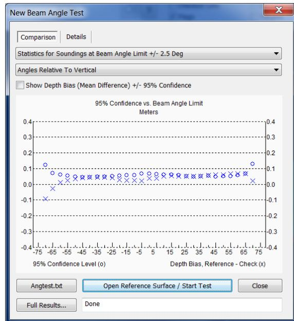
**FIGURE 3.** New BAT using beam angles in the sonar frame. A hybrid between the original test and the new one.
