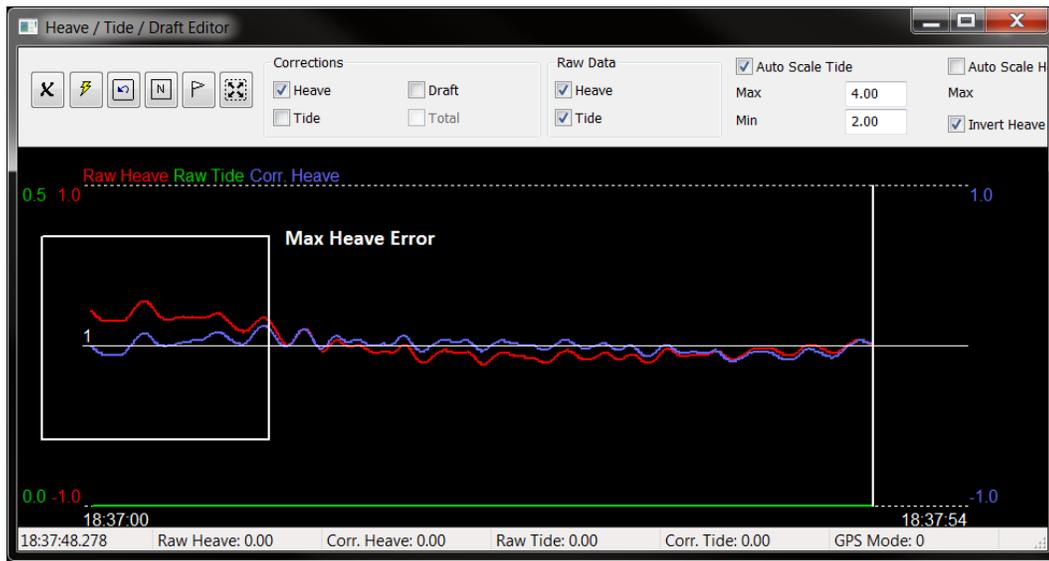
**Figure 5** shows an along track depth profile, with and without delayed heave. There's the 10 cm error at start of line.
