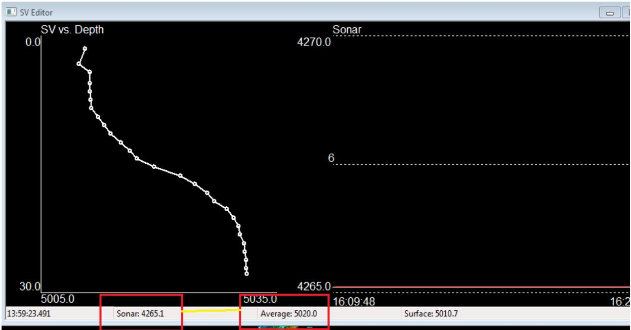
When overlaying the post-dredge survey, which has a good sound velocity entered, and the pre-dredge survey, the shift is a vertical difference of over 4 feet!
