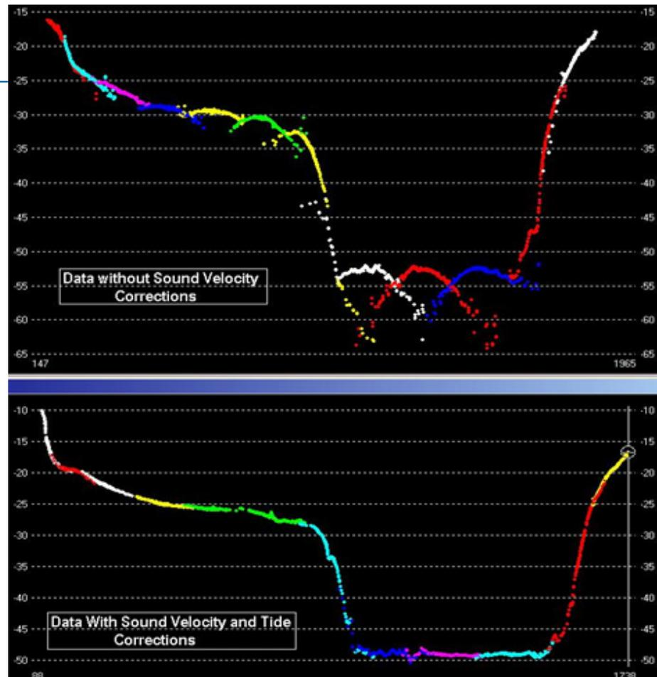
Here is what we finally saw with the data: There was no real-time sound velocity of the head. It was manually entered into the sonar as a static number. When comparing the cast data for that day and the probe sound velocity, we see a 755 ft/sec difference from the value entered in for the sonar and what the cast data showed. Notice the sound velocity at the Head (4265.1) vs. Cast (5020.0)
