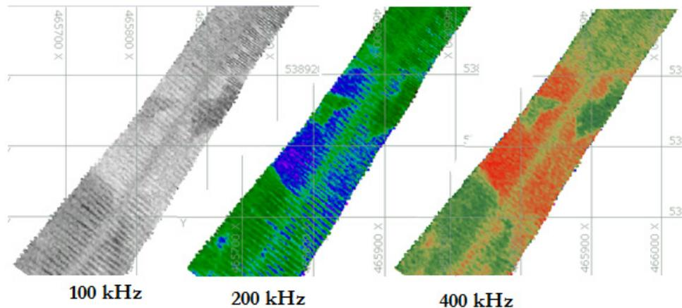
This third item bears further explanation. Systems like the R2Sonic 2026 now offer a multispectral mode which allows the MBES to frequency hop between pings, enabling you to collect data from three distinct frequencies in a single pass. The HYPACK® data converter can bring this data in, but we'll improve the collection and processing tools this year. By
