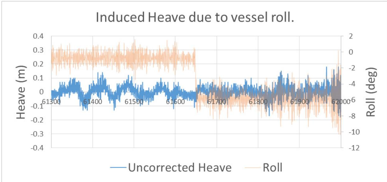
If we have properly corrected heave, then the zero point does not move with the change in the draft of the sonar and that increase in the draft is properly measured. Figure 4 shows what the heave signal looks like when this occurs. When the roll occurs, we see a simultaneous shift in the heave indicating an increase in the draft of the sonar.
