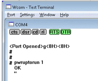
**IMPORTANT:** Once the 'pwruprun 1' command is sent to the EXO Sonde, it will be stored in the memory of the SOA-DCP, therefore, the Sonde will immediately start transmitting data upon 'Power Up'.
