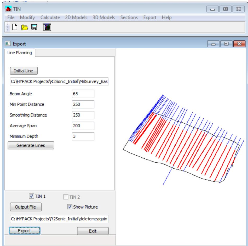
The resulting planned line may require some additional processing inside the LINE EDITOR. For example, I have extended some lines and clipped them inside the BRD file to better fit my survey area.
